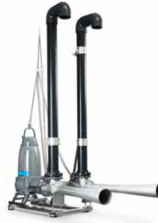
The Flygt jet aerator consists of air suction pipes, an N-pump, ejector housings and ejectors.
