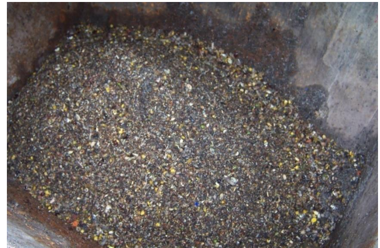
Typical unwashed grit trap material
