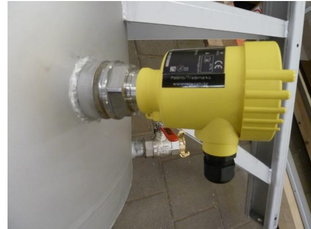
Capacitive pressure probe – real-time measurement
