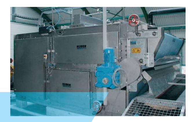
Belt filter press for municipal and industrial sludge High-performance belt filter press for best dewatering results Combi-unit: thickening and dewatering in one working process
