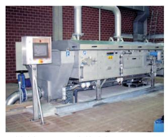
Drainbelt for up to 100 m<sup>3</sup>/h thin sludge
