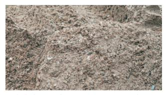
Washed grit removed at a wastewater treatment plant
