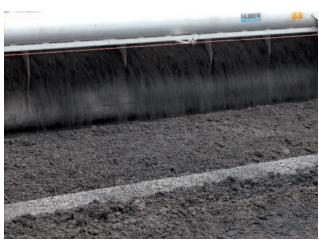
Backmixing and aeration of sludge
