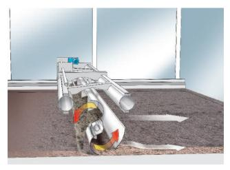
The rotating shovel of the sludge turning and mixing device takes up sludge and transports it along the granulation plate. As the turning device travels forward, the sludge is transported.
