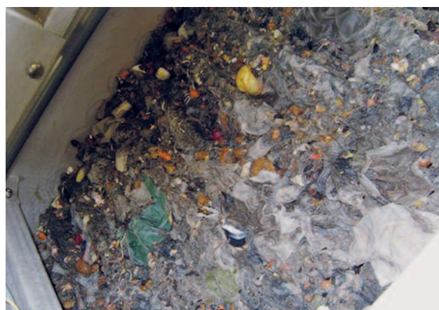
STEP SCREEN® Flexible: high separation efficiency due to the narrow slot width and the produced screenings carpet, self-cleaning effect due to a moveable lamella unit.
